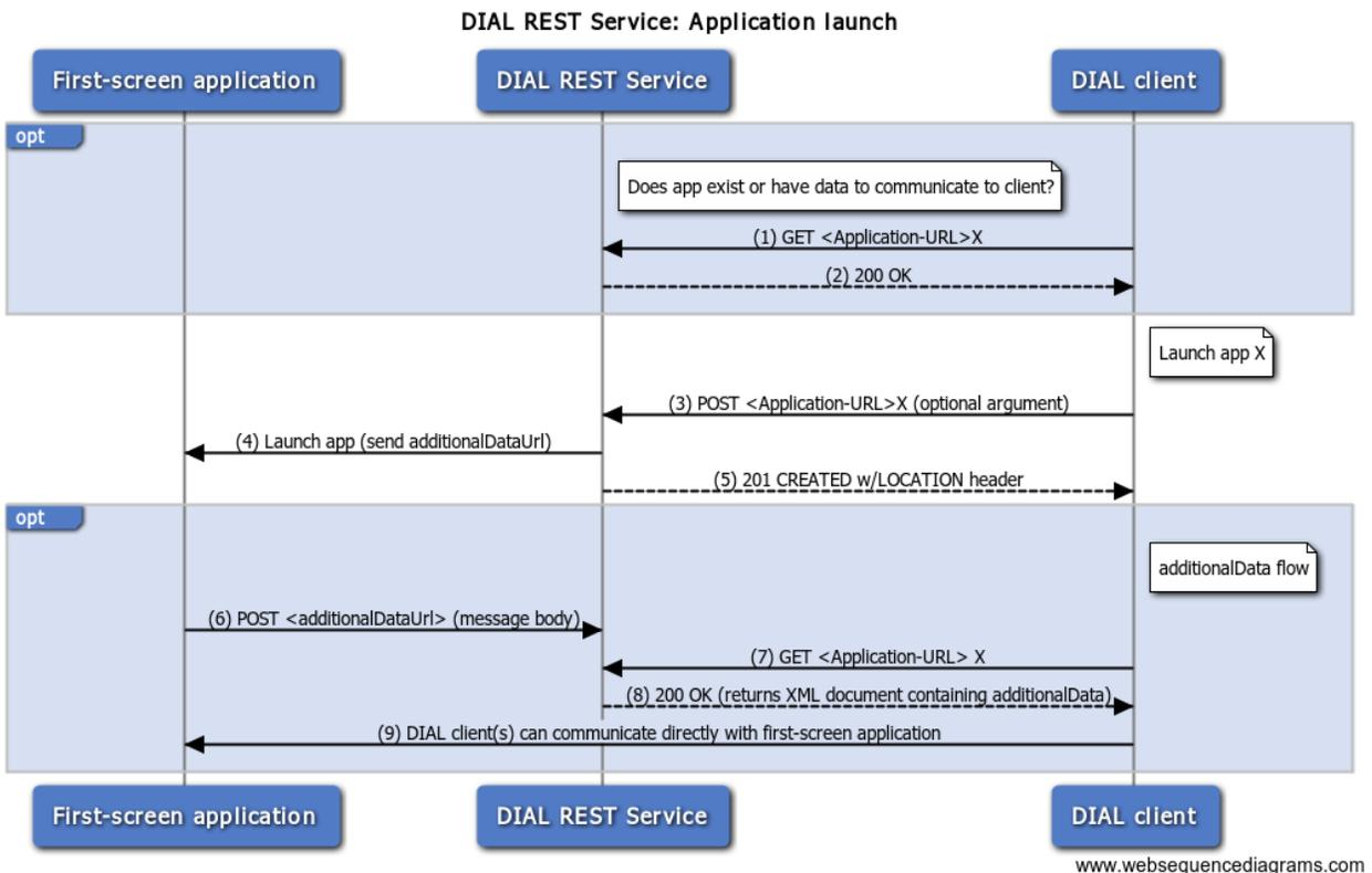
The process diagram above illustrates the process by which a first-screen application can send data back to the DIAL server. The DIAL server can subsequently communicate to any second-screen device that contacts it. The following notes explain the image in more detail:
